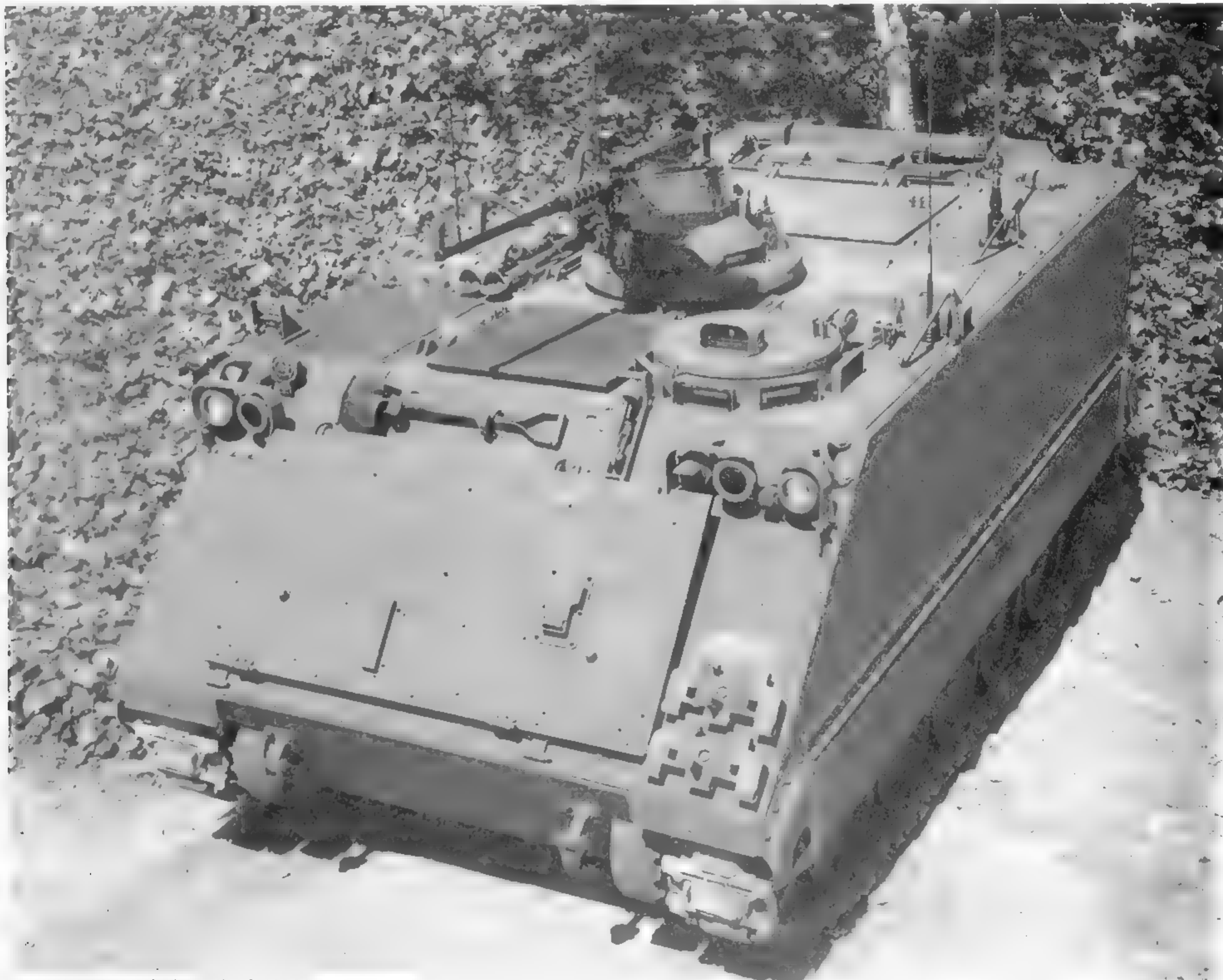
While in this basic form the M113A2 looked much like its predecessor, it had the capability to use rear-mounted external fuel tanks instead of the traditional internal ones. (U.S. Army photo)
